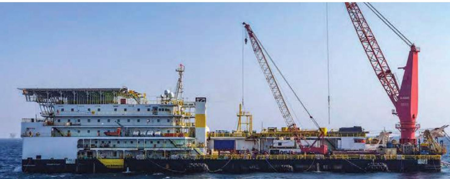
*LTB 300, a pipelay-cum-work barge undertaking offshore installation*
