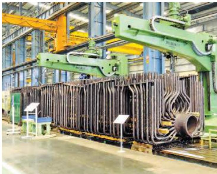
Boiler internals being manufactured at Hazira, Gujarat
