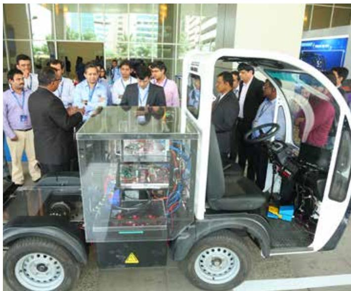
*LTTS prototype of the Battery Management System used in Electric Vehicles*
