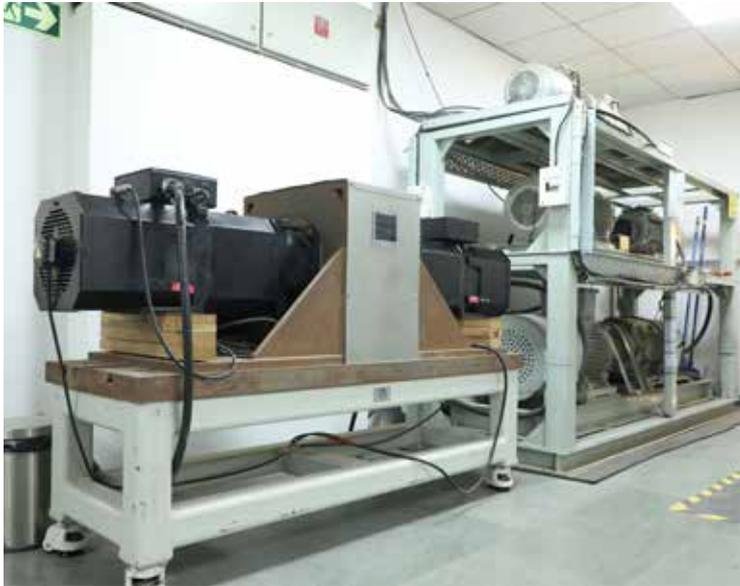
*LTTS' Motor Dyne system conducts troubleshooting of power electronics*
