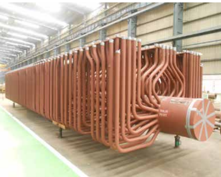
Supercritical boiler internals being manufactured at Hazira, Gujarat
