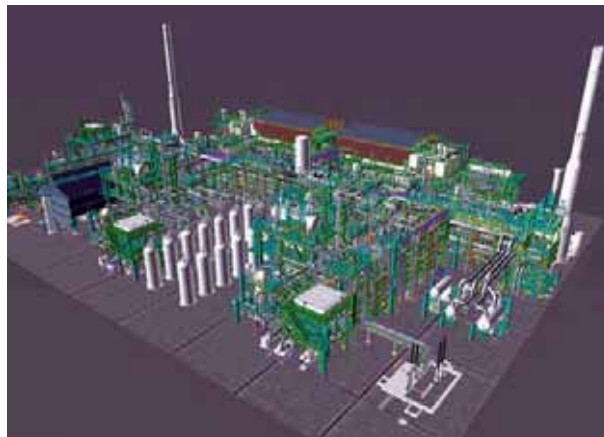
3-D CAD model for 2 x 44,000 MTPA Hydrogen Generation Units for Guru Gobind Singh Refinery of HPCL-Mittal Energy at Bathinda (Punjab).
