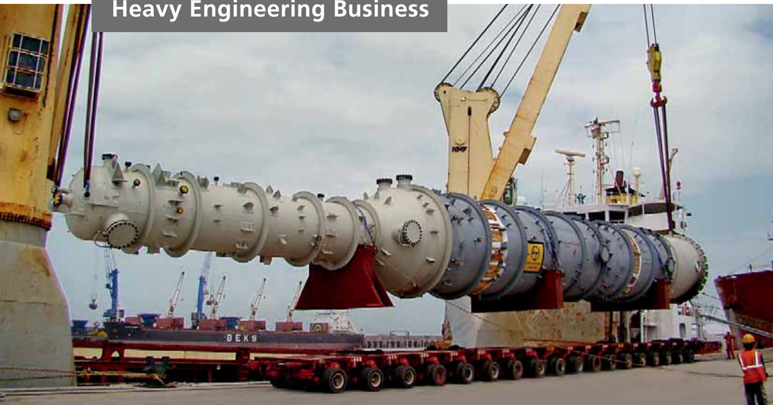
A low-alloy steel HP stripper being shipped from L&T's Hazira Campus to a refinery in Texas. L&T has designed, manufactured and supplied critical process plant equipment to over 40 countries.
