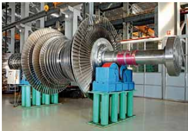
Supercritical turbine being assembled at the Hazira Campus.
