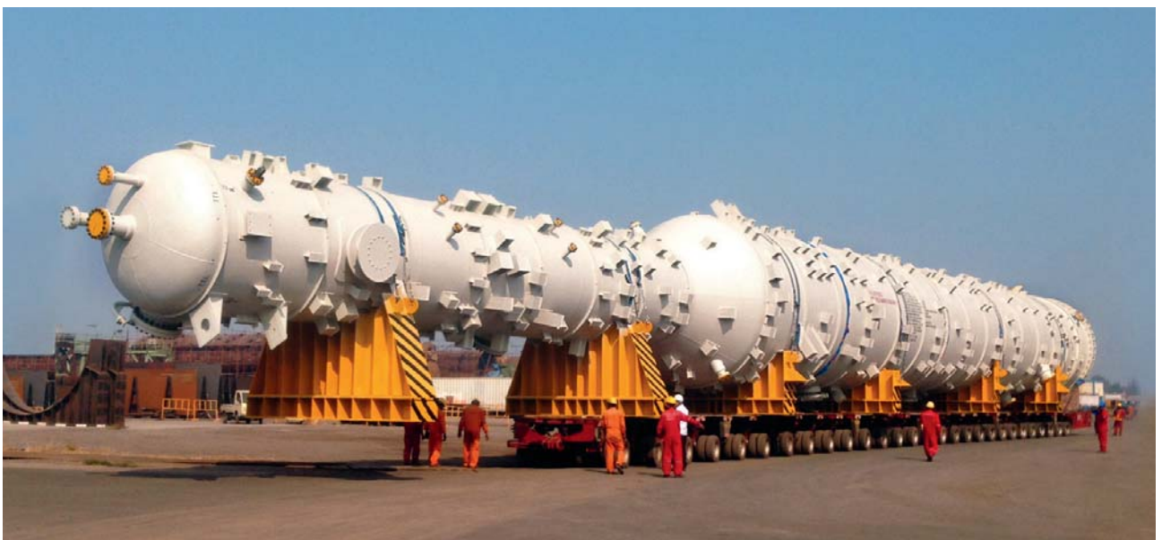
Unsaturated Gas Demethanizer. L&T has designed, manufactured and supplied critical process plant equipment to over 40 countries
