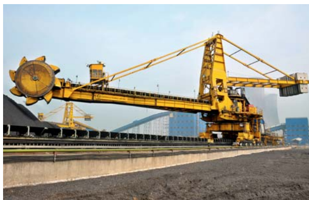
3600 TPH Stacker Reclaimer, Rajpura, Punjab. One of the many industry-wide bulk material handling solutions provided by L&T
