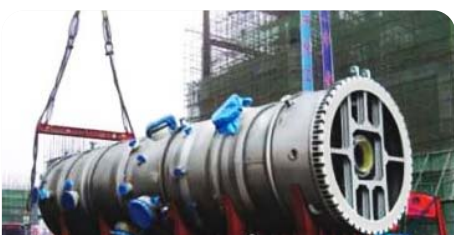
Coal Gasifier for China
