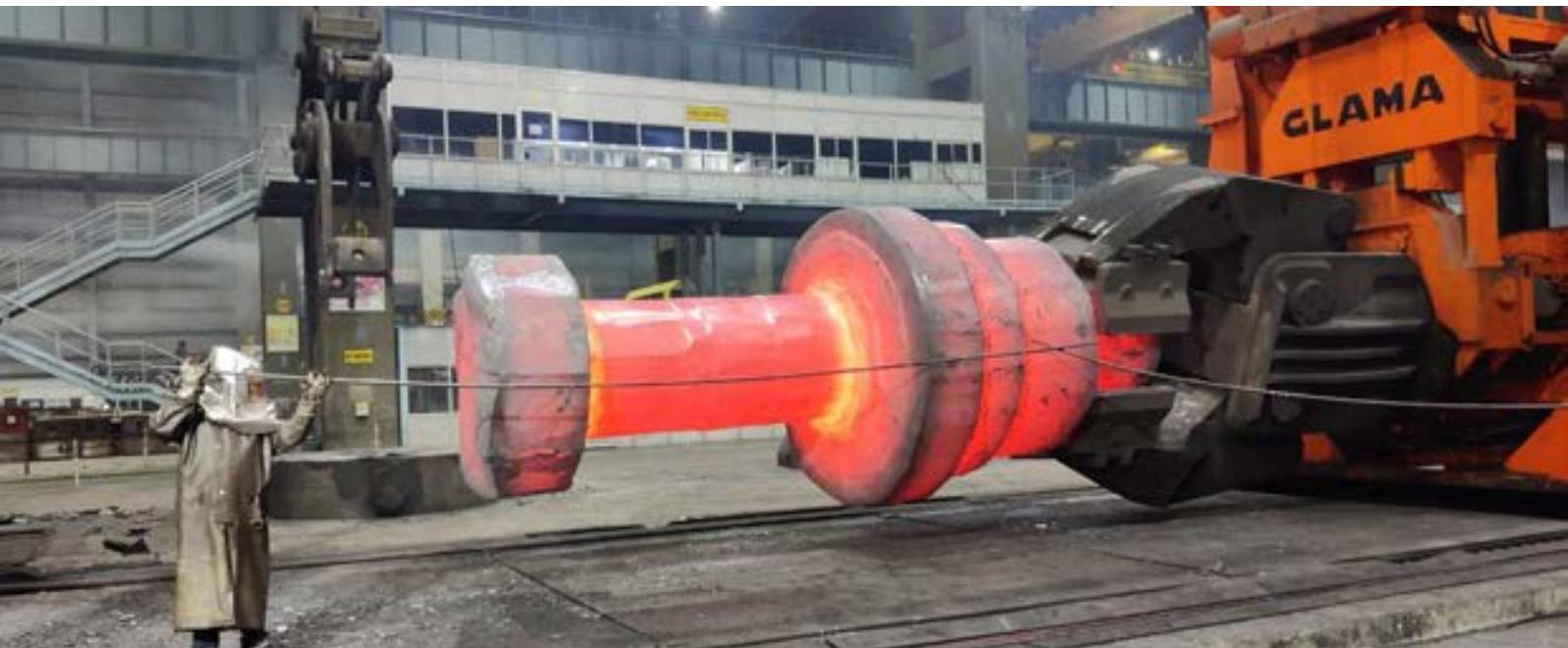
Forged Hydro Shaft, weighing 36 MT, for BHEL
