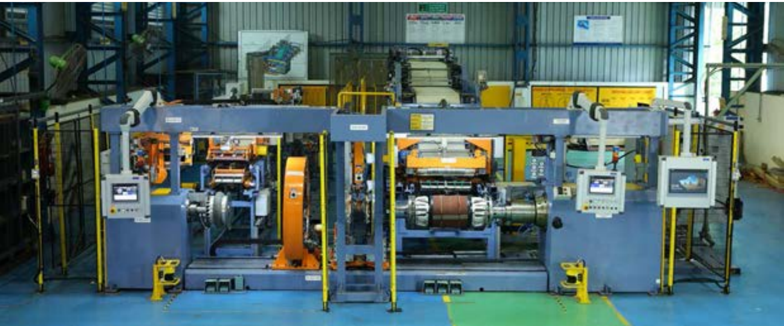
Motorcycle radial tyre-building machine
