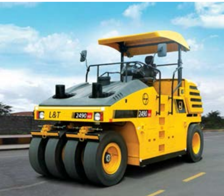
L&T 2490 Pneumatic Tyred Roller is increasingly preferred by contractors to seal surfaces and achieve a smooth finish
