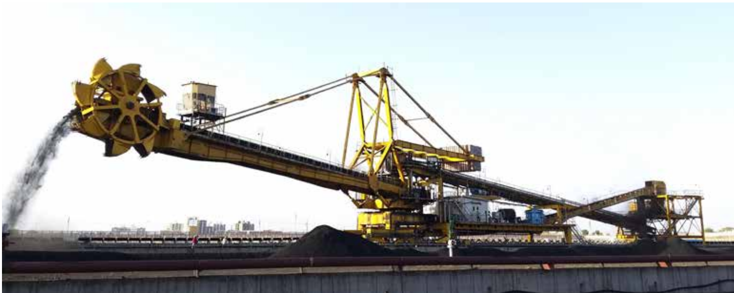
7C Stacker-cum-Reclaimer installed at Khargone
