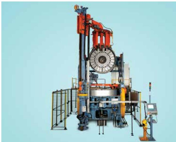
OTR Mechanical Tyre Curing Press
