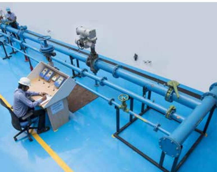
R&D Facility – Flow Co-efficient Test
