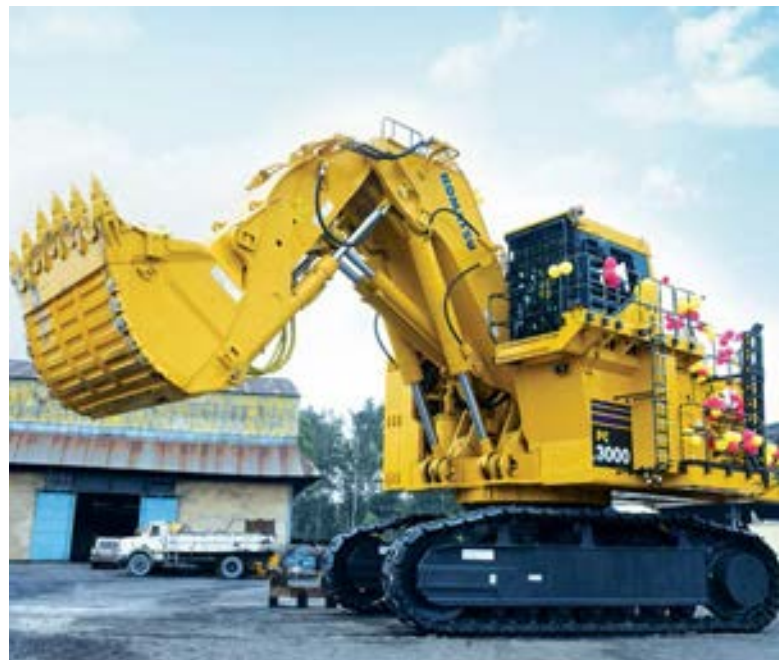
L&T ushered in mega mining with supply and commissioning of PC3000, Komatsu's first 300-ton Electrical Shovel in India, at South Eastern Coalfields Limited, Gevra Mines
