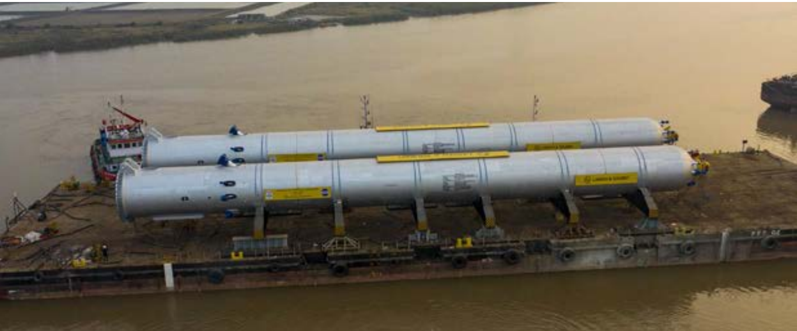
The world's heaviest LC MAX Reactors, weighing 2313 MT, on the way to HPCL, Vizag
