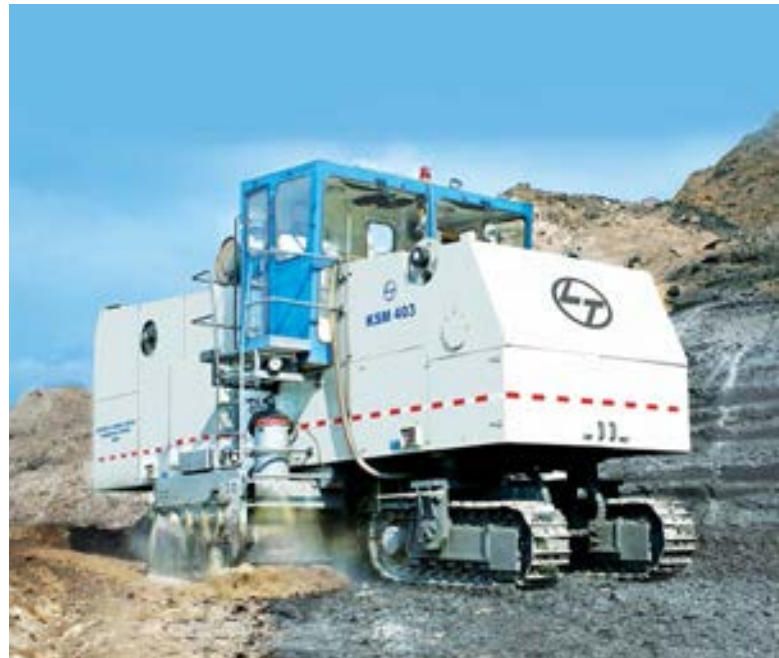
KSM 403 Surface Miner – indigenously designed and manufactured by L&T for eco-friendly and sustainable mining in open cast projects.
