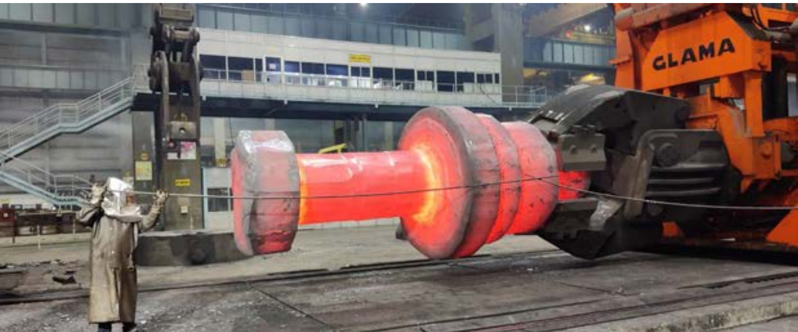
Forged Hydro Shaft, weighing 36 MT, for BHEL
