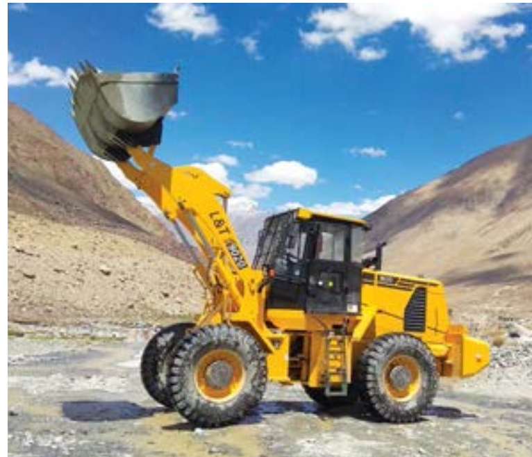
L&T 9020 Wheel Loader deployed by Border Roads Organization to construct and upkeep strategic roads and border infrastructure
