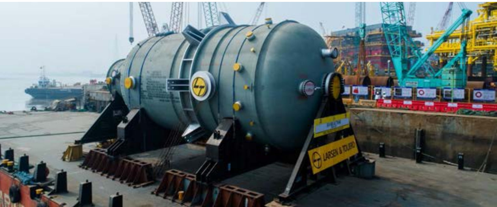
Ethylene Oxide Reactor weighing 1157 MT for IOCL's Paradip Refinery
