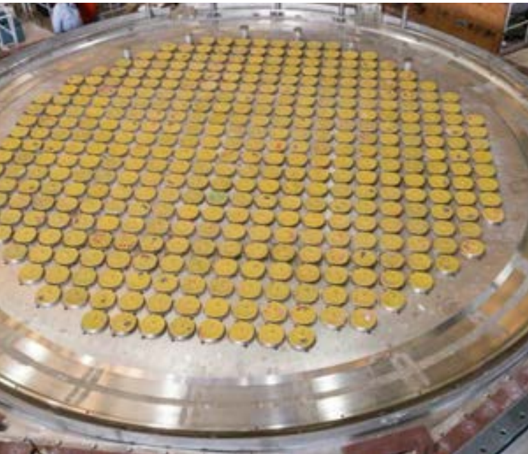
End Shield for the 700 MWe Nuclear Power Plant – GHAVP
