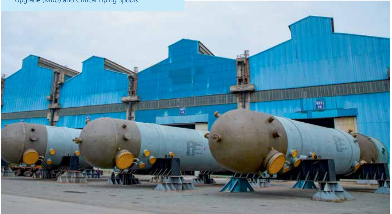
Propylene Oxide (PO) Reactors
