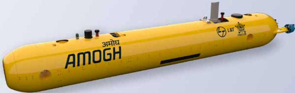
L&T's AMOGH - Autonomous Underwater Vehicle for surveillance
