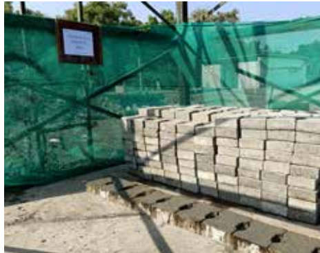
Paver Blocks from concrete waste
