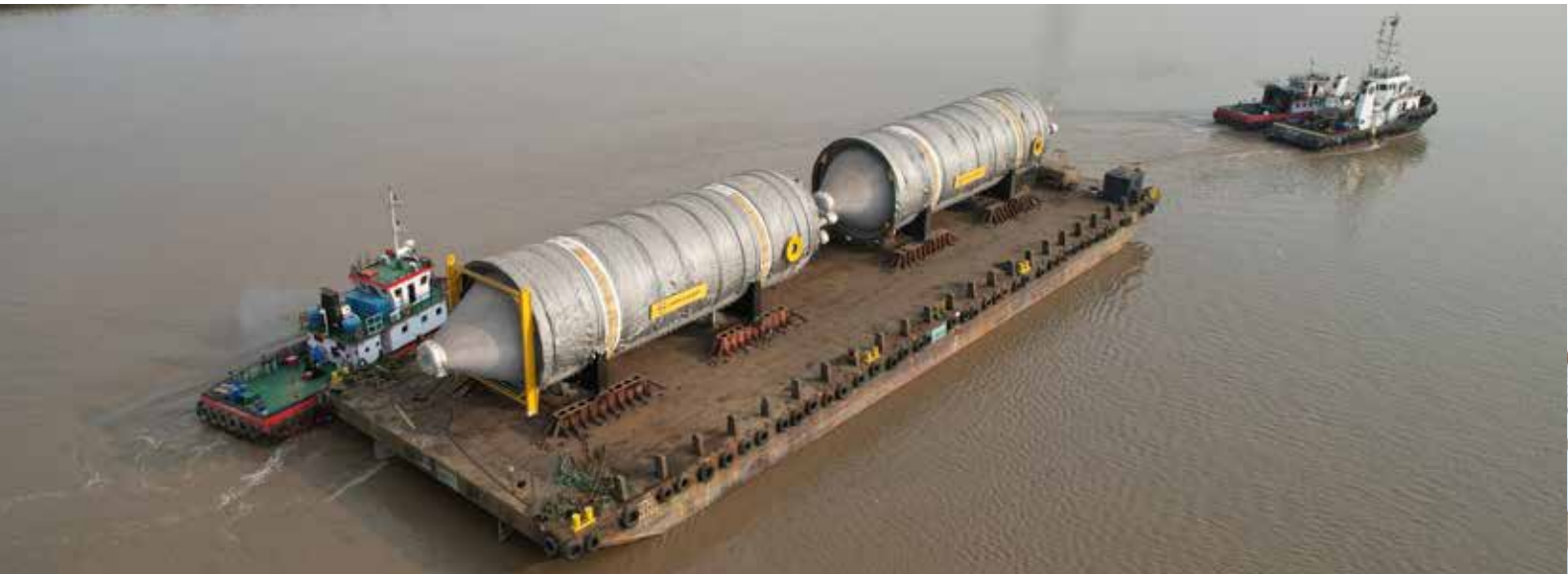
Coke drums each weighing 450 MT for Numaligarh Refinery Limited, Assam
